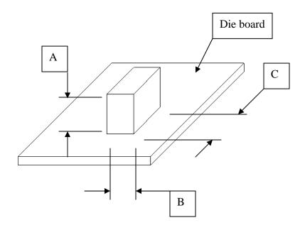
Example: When ordering a block with a 5/8" height, 7/8" width, and 1 1/4" length, specify as follows:
